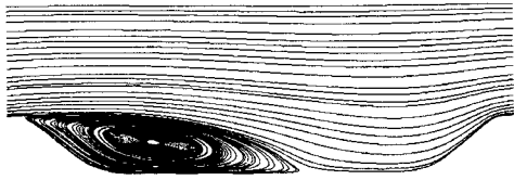
Figure 3: Stream streaks for turbulent flow over a periodic hill at Re=10595 .
