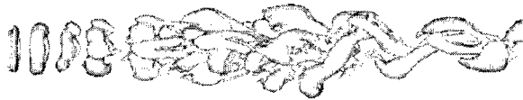
Figure 5: Spatial evolution of coherent vortices shown by isosurface of positive Q for the natural jet at Re = 36000 , M = 0.7 and t = 30D/(U_1 - U_2) .
