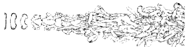
Figure 3: Isosurfaces of Q criterion for the natural jet at Re = 2000 , M = 0.7 and t = 300D/(U_1 - U_2) .
