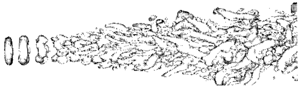
Figure 4: Isosurfaces of Q criterion for the natural jet at Re = 25000 , M = 0.7 and t = 300D/(U_1 - U_2) .
