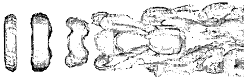
Figure 7: Visualization of the streamwise hairpin vortex by isosurfaces of Q criterion for the natural jet at Re = 36000 , M = 0.7 and t = 100D/(U_1 - U_2) .
