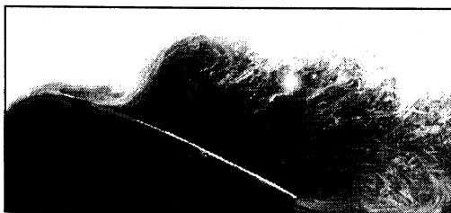
Figure 2. Phase-averaged image during the reattachment process.
