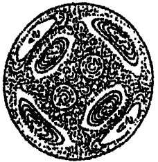
Figure 1. Mixing in a steady, spatially periodic flow. Figure (a) shows a typical Poincaré section, with the numbers indicating the period of the islands; figure (b) shows the typical three-dimensional structure of the system. Note that the fluid within the KAM tubes does not mix with the rest of the fluid. From Khalash et al. (1987).
