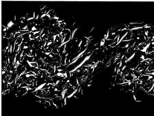
Figure 9: Isosurfaces of the second invariant (white) and energy dissipation rate (gray) at t = 130 ( Re_{\omega,0} = 700, Q^* \geq 0.01, \epsilon \geq 2\epsilon_m ).
