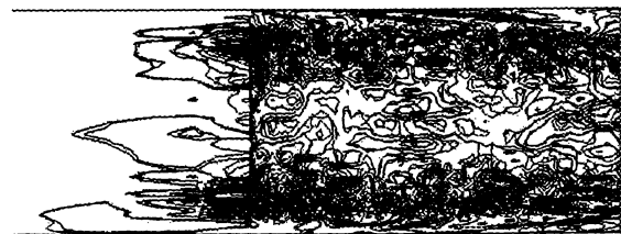
Figure 8: Development of spanwise velocity showing initiation of unsteady motion in refined-grid region
