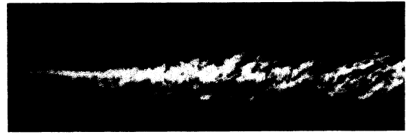
Figure 7 : Instantaneous schlieren image of M_c = 1.7 mixing layer case. Imaged region is 23 x 8 cm. s = 1.57 , r = 0.02 .
