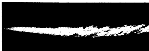
Figure 3 : Instantaneous schlieren image of M_c = 0.8 mixing layer case. Imaged region is 23 x 8 cm. s = 0.23 , r = 0.07 .
