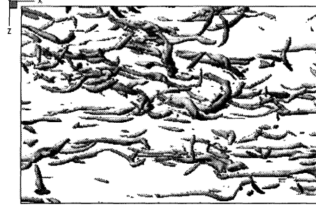
FIGURE 12. Vortices in channel with spanwise moving wall at t^+ = 13.5 : symbols same as in Figure 10.
