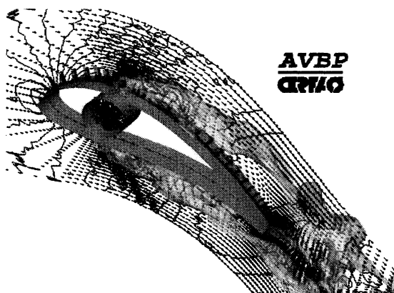
Figure 10: fuel injection on a part of the vane, isosurface: mixture fraction, isocontours: pressure, black arrows: velocity vectors
