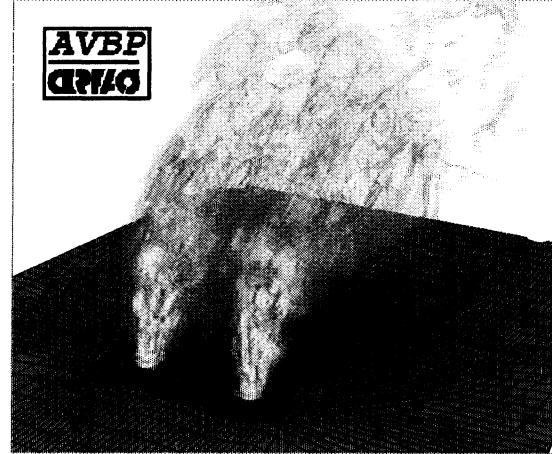
Figure 8: smoke vizualization of the testcase of Toy, r = 6 , Re=31800
