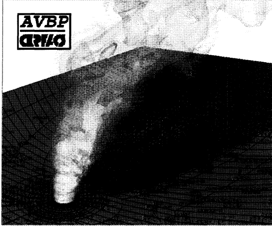
Figure 6: smoke vizualization of the testcase of, Smith & Mungal, r = 5 , Re=16400
