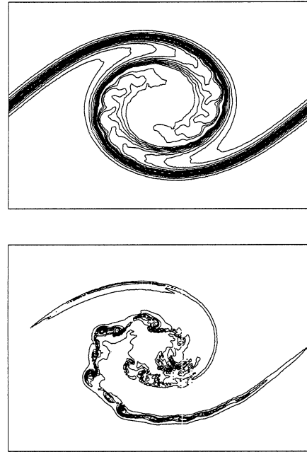
Figure 3: Iso-vorticity contours at t = 20.0 for temporal mixing layers. Case I : uniform density, Case II : variable density ( \rho_1/\rho_2 = 3.0 )
